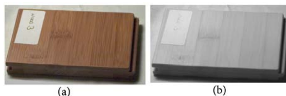
Figure 1: A typical photograph from a wood sample in the a) visible b) NIR part of the spectrum. The colorant is transparent to the NIR and intrinsic texture is observed.
