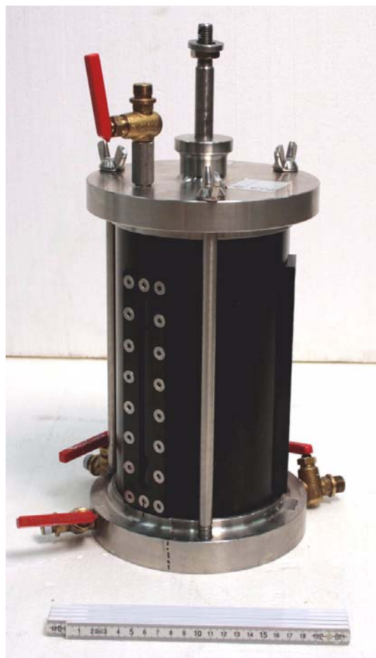
Fig. 3.17. Triaxial cell mounted with the aluminium walls and glass windows.
