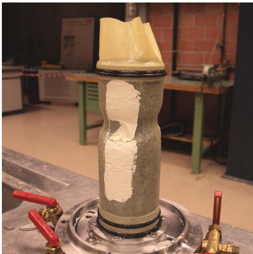
Fig. 4.52. Strain localization of a Lemman Sand sample (paint layer in white for laser measurement).
