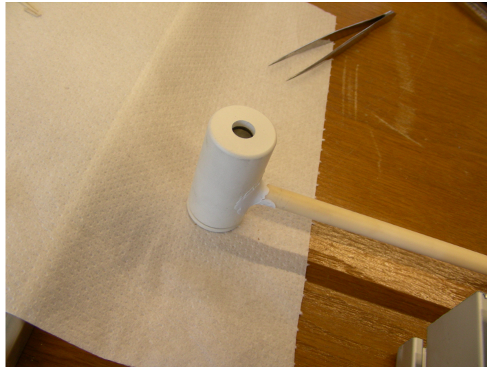
Figure 4.13: The incased fast ion source.
