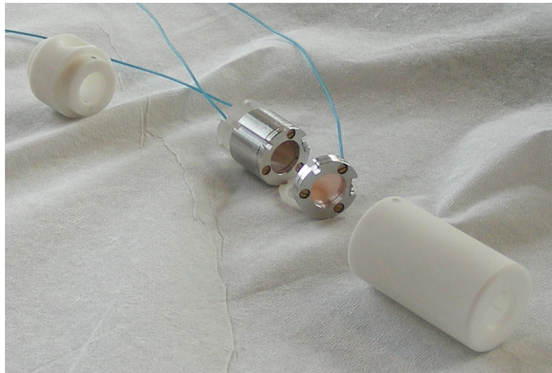
Figure 5.3: Assembling one of the two identical parts of the detector. The macor casing and the grids squeezed between aluminum rings can be seen.
