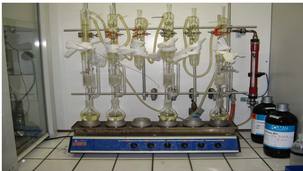
Figure 4.2: Soxhlet extraction system used for PTSs analysis
