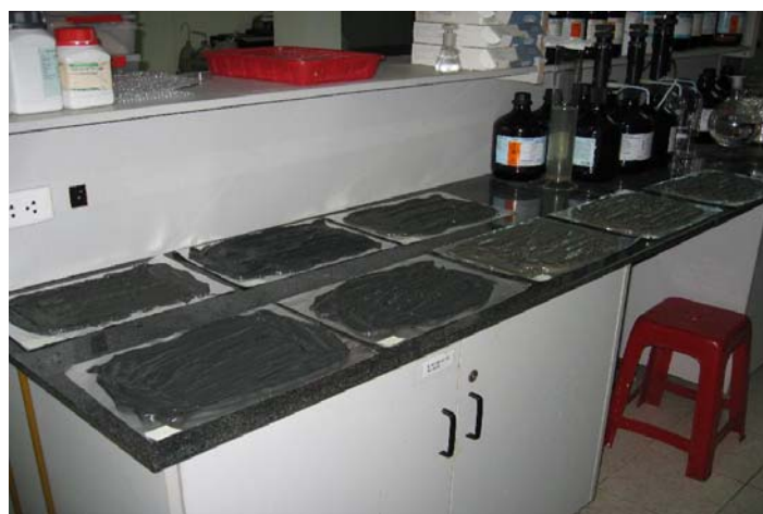
Figure 5.10: Drying sediment samples in IER laboratory
