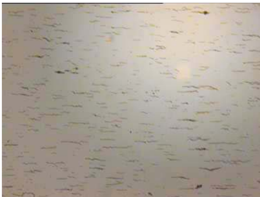
Figure 1. Magnetic beads ( 1 \mu\text{m} ) in a permanent magnetic field with a low field gradient.
