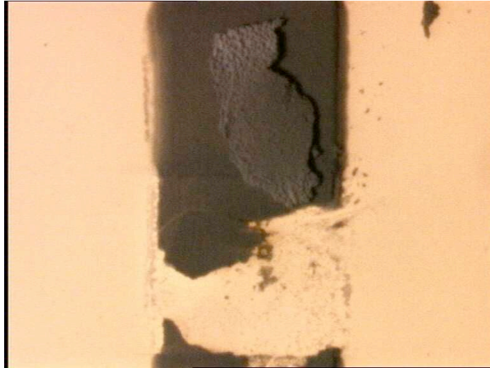
Heraeus GPA 98-029 (left) & ESL 4924 (right) after \approx 1 day in acid Failure in 10% acetic or phosphoric acid @ RT
