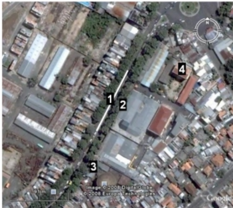
Figure 4.1. Measurement site. 1: Emission liberation device over the Ba Thang Hai street. 2: mobile station. 3: traffic video recording. 4: Meteorological station. Adapted from Google earth.
