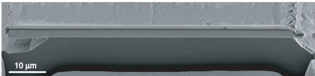
Figure 4.15: SEM image of a FIB cross-section of the double resonator structure on MgO. The resonator was cut in-between the two resonators of the double resonator structure.
