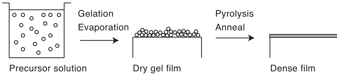
Figure 2.2: Principle of the sol-gel process.
