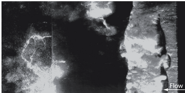
(a) Leading edge cavitation (Naca0009, \alpha=4.5^\circ , C_{ref}=14 m/s, \sigma=1.2 )
