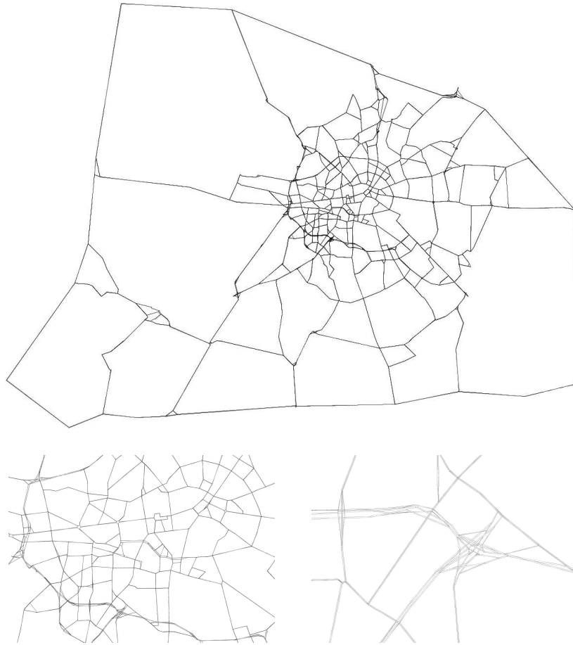
Figure 2: Major road network of Greater Berlin The network consists of 1 083 nodes and 2 459 unidirectional links. The two clip- pings indicate a locally high modeling resolution.
