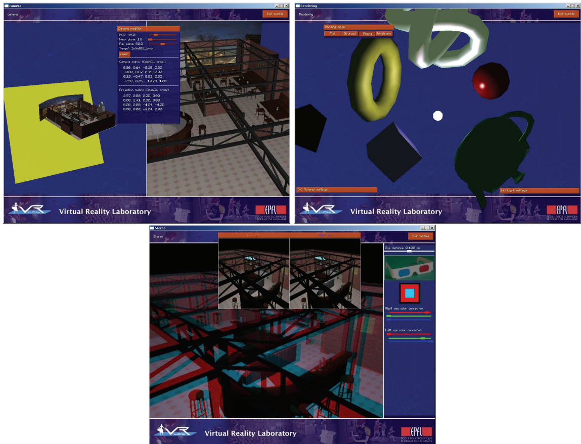
Figure 5.8: Camera handling (top left), shading techniques (top right), and stereographic rendering modules.
