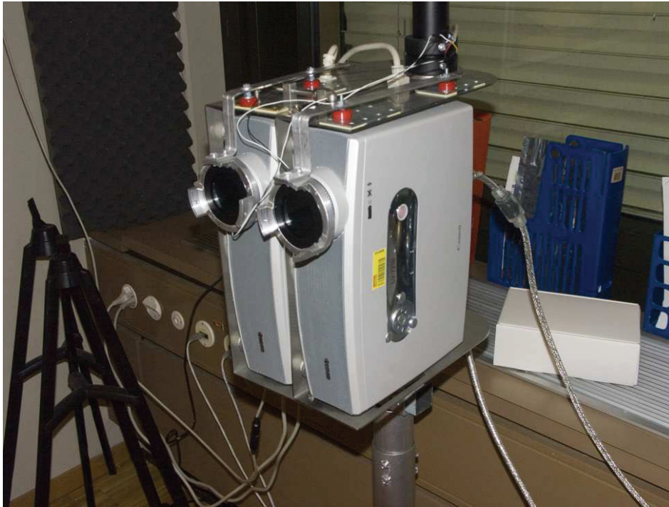
Figure 5.13: Dual-projector assembly with shutters.
