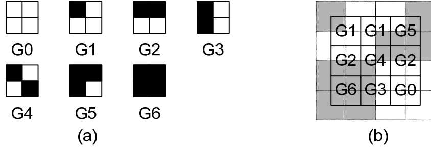
Fig. 2. (a) The 7 calibration patterns for the black and white 2-by-2 model. (b) Example of a halftone with the corresponding mapped 2-by-2 patterns.
