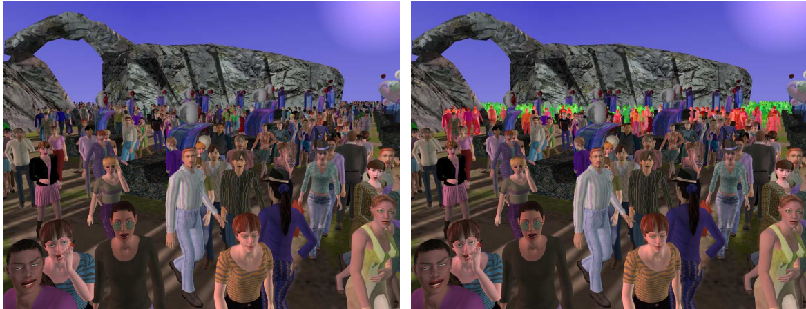
Figure 7.6: ( left ) Virtual humans navigating in a complex environment. ( right ) Same configuration of virtual humans with apparent levels of detail; in red: the rigid meshes, in green: the impostors.
