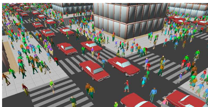
Figure 2.11: In [Treuille et al., 2006], crowds are steered by a potential field to reach their goals while avoiding collisions.
