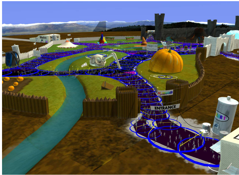
Figure 10.1: A navigation graph is composed of circles representing navigable areas. When two circles intersect, pedestrians are allowed to navigate from one navigable area to the other.
