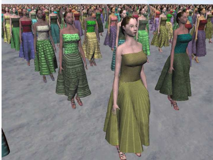
Figure 2.8: The physical simulation of clothes is pre-computed and re-used on rigid meshes and impostors [Dobbyn et al. , 2006].
