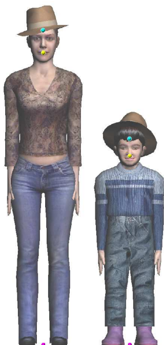
Figure 5.1: Two human templates wearing the same hat, in their default posture. The pink, yellow and blue points represent the position and orientation of the root, the head joint ( m1 ), and the hat accessory ( m2 ), respectively.
