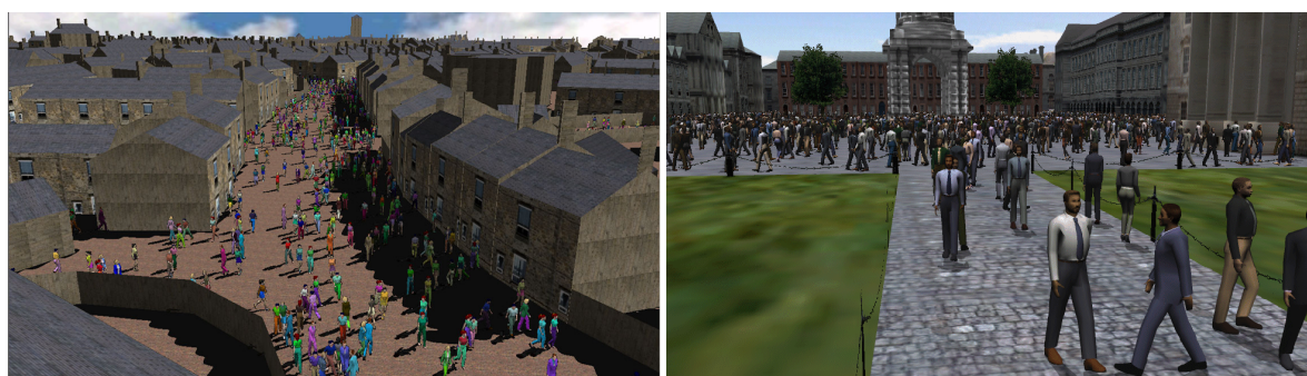
Figure 2.1: (Left) The use of billboards allows Tecchia et al. to simulate large crowds [Tecchia et al., 2002a]. (Right) Dobbyn et al. combine static meshes and billboards to have a higher quality rendering in front of the camera [Dobbyn et al., 2005].
