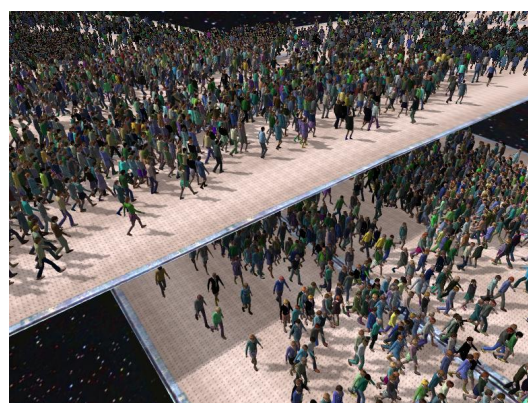
Figure 3.10: (Left) A Navigation Graph has been computed for the planet eight environment, and a single starting/destination points were input. (Right) The slopes in the environment are sufficiently gentle to allow the crowd to move on them. The two levels of the environment are correctly handled by the Navigation Graph [Pettré et al., 2006].
