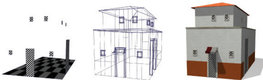
Figure 6.5: A building contains invisible geometry (checkerboard) which is used to store the semantic information.
