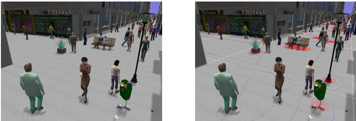
Figure 7.1: ( Left ) A procedurally generated pedestrian street, successfully populated with crowd patches. ( Right ) The same image showing apparent pre-computed trajectories and patch borders.
