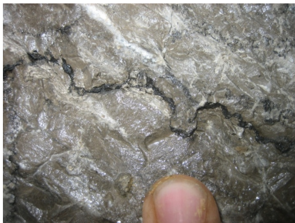
Fig. 3.25: Stylolite in a Jurassic limestone. Although some similarities stylolites (wave-like interlocking surfaces that contain concentrated insoluble residue such as clay minerals and iron oxides) should not be confused with dissolution seams (i.e. touching vugs).
