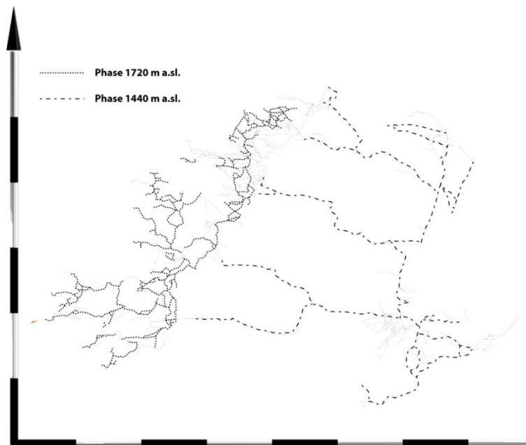
Fig. 2.11: Plan view of the Siebenhengste Cave System with a rose diagram of the conduit directions of the phase 1720 and 1440: The directions of the conduits are dominated by the fracture network as well as by the hydrogeological boundary conditions. The change of the hydrogeological boundary conditions between the two phases caused the preference of another set of fractures.
