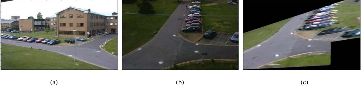
Fig. 6: (a) First view, (b) Second view, (c) Homography transform of the first view to the second.
