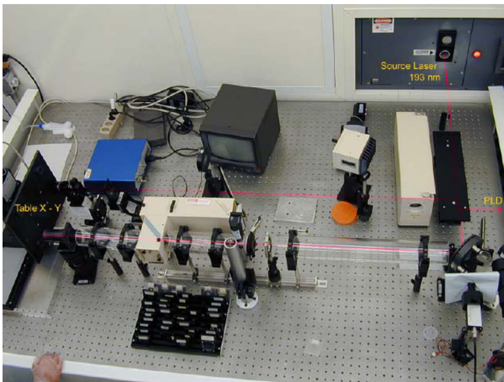
Figure 3. A photographic view of the excimer laser ablation system used.
