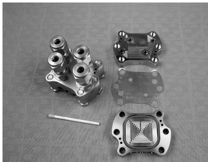
Fig. 5. Type 3 microstructure reactor for thermal unsteady state running of chemical reactions.
