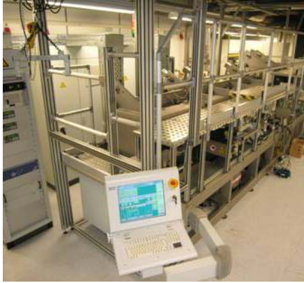
Figure 2: New MW-PECVD roll-to-roll system built by the system manufacturer R&R and shipped to ECN
