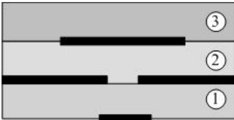
Fig. 3 SSFIP antenna geometry
