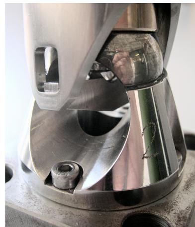
(b) Close-up on the contact region and the preloading system. The preload is applied on a smaller ball, by this reducing the friction by a factor 3 in the preloading system.
