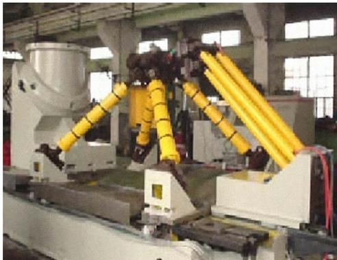
(a) The 5-axes parallel-kinematic machine tool proposed by Feng Gao.
