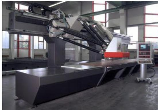
**Figure 4.14:** The Pegasus basic concept with 3 DOF in translation. This version is a purely parallel kinematics.
