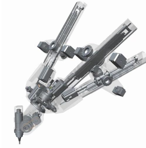
(a) Image of the Exechon machine tool. A 5-axes hybrid kinematics for machining tasks.
