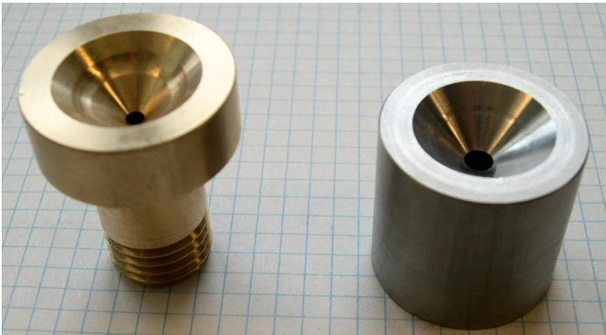
**Figure 6.12:** Picture of two cones (bronze-alloy and steel, for a 15mm ball) after a stamping of 50kN on a hydraulic press. The stamped surface is visible as a ring on the cones.
