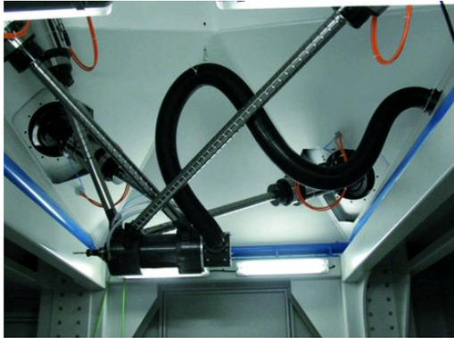
(a) The Metrom parallel kinematic machine. (www.metrom.com)
