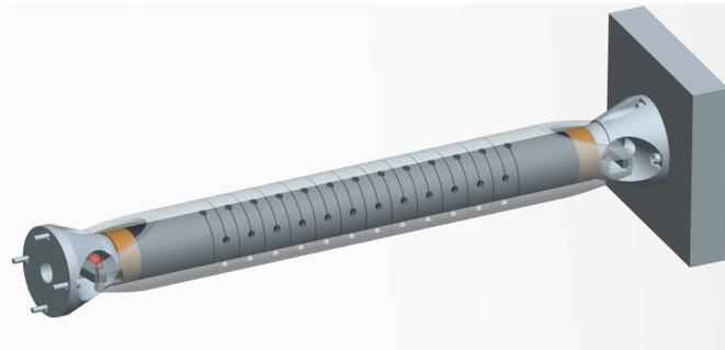
**Figure 9.5:** Strut with 2 modified first-evolution spherical joints sharing a common preloading system. This system consists of an elastic tube which has been partially cut, in order to obtain the required preloading force.
