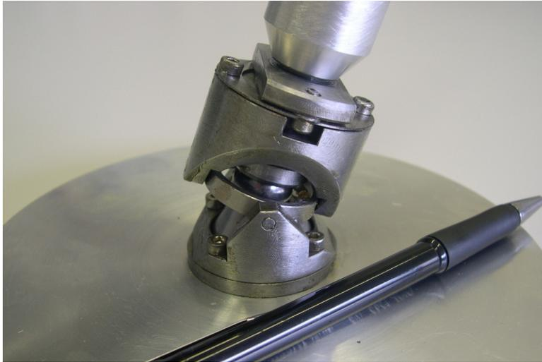
**Figure 6.16:** 3rd evolution of the spherical joint. First concepts of this type of joint were proposed in June 2004 (45).
