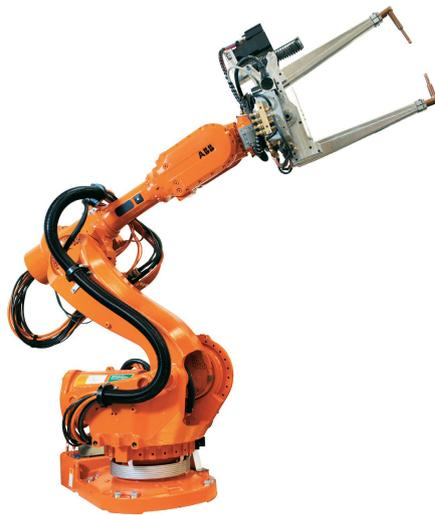
(a) A serial-kinematic robot from ABB.
