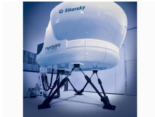
(b) Variable strut-length drive system on a flight simulator from Sikorsky ([www.sikorsky.com](http://www.sikorsky.com)) at the FlightSafety ([www.flightsafety.com](http://www.flightsafety.com)) facilities. The 6 identic struts synthesize a parallel kinematics called **Stewart platform**. One of these legs is represented in the kinematic scheme on the left.**Figure 4.25:** The variable strut-length drive system.
