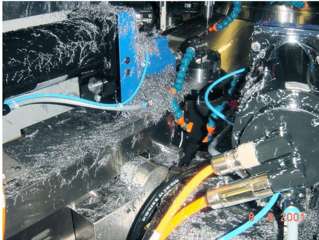
**Figure 7.6:** Inside view of a machining center. Chips can be found everywhere, and will go everywhere you thought they wouldn't!
