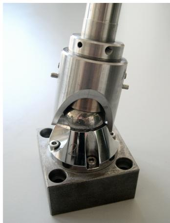
(a) Picture of the 1st evolution spherical joint. The spherical surfaces are machined in the basic components of the joint, therefore leading to relatively complicated parts
