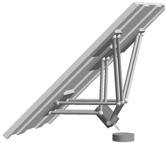
(b) A model of the 4 parallel axes of the Hita STT.
