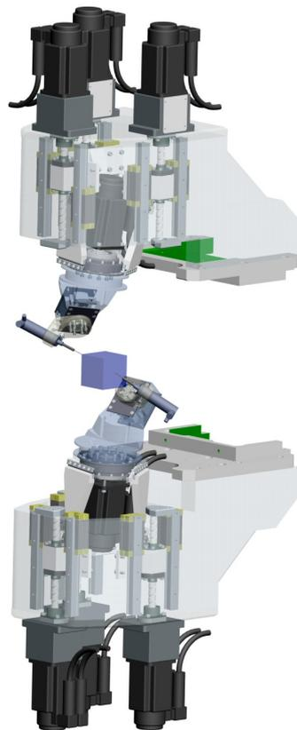
**Figure 9.21:** Example of 2 modules working on the same setup. The way the 2 modules are arranged allows to cover the complete angular range (complete sphere). The cube in the center represents the working volume of the modules.
