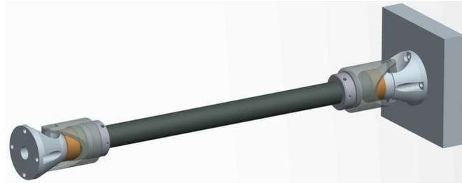
**Figure 9.4:** Simple bar with 2 separated first-evolution spherical joints.
