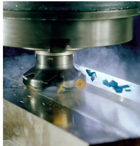
(b) Milling machine during a surfacing process (picture by [www.epma.com](http://www.epma.com))
