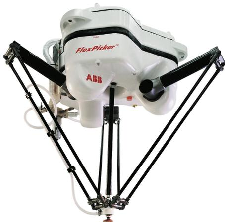
(a) The ABB 360 Flexpicker, a 4-axes, hybrid kinematics for high-speed pick-and-place applications.
