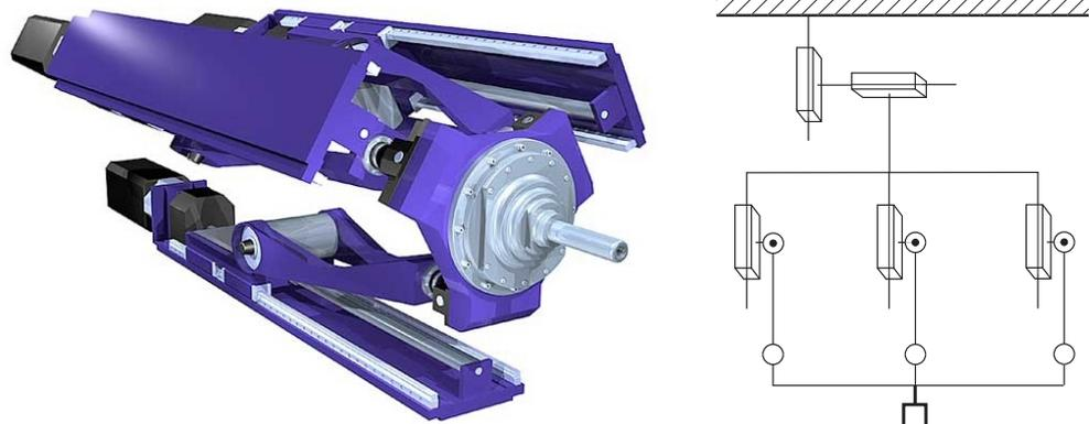
(a) Image of the Sprint Z3 Head. This module has 3 DOF, 1 translation and 2 rotations. It is used in combination with 2 serial axes for translations, by this constituting the ECOSPEED 5-axes machining center.
