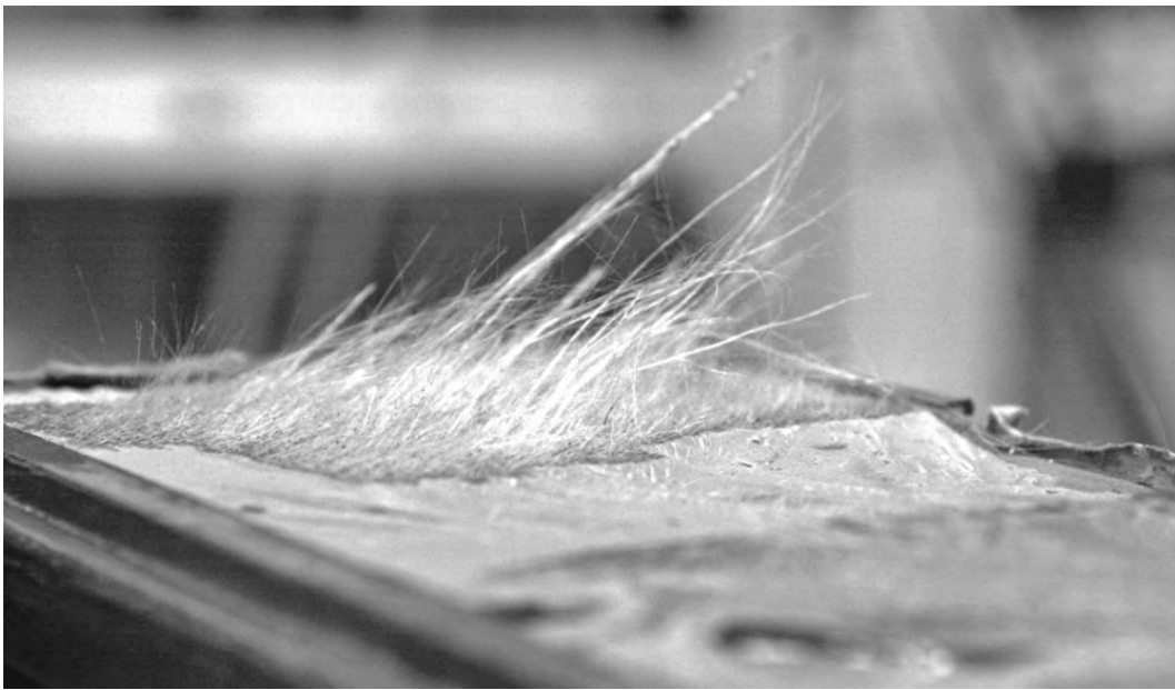
Figure A.14: Fiber-tear failure on surface and adhesive failure (C3-1)
