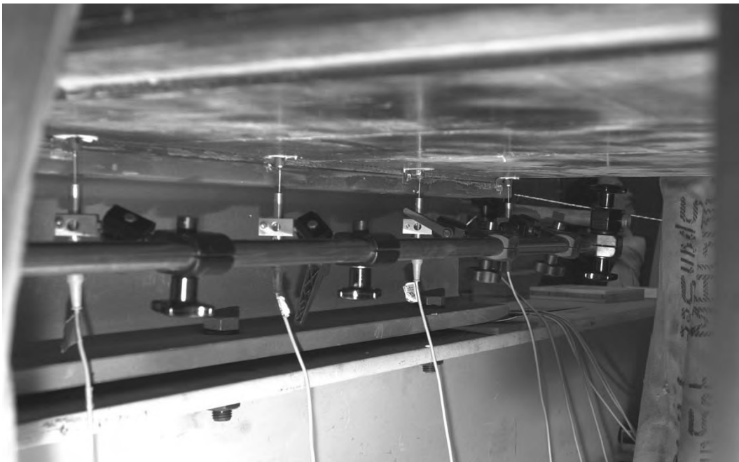
Figure 3.17: Displacement transducers measuring deformations at adhesive bond between edge of bridge deck and steel girder on inner side
