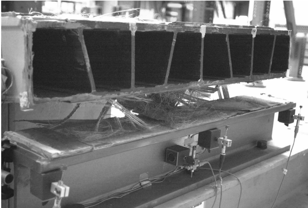
Figure A.9: Failed adhesively-bonded connection (C2-2)
