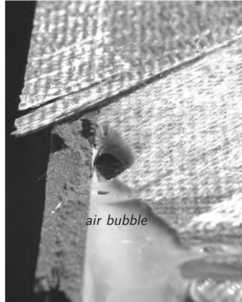
(b) Air bubble near to the edge
