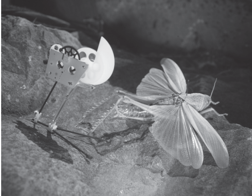
Fig. 11 7 g jumping robot prototype capable of clearing obstacles of up to 1.4 m height along with a desert locust using the same biomechanical design principle for jumping.
