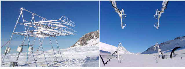
FIG. 8. (Color online) Side view of the SnoHATS setup of sonics arrays (left) and upwind fetch (right).
