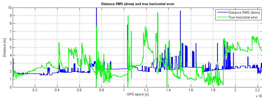
Figure 4.9: True horizontal error and drms estimation provided by the receiver.
