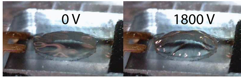
Figure 6.21: Left: picture of a \varnothing 3 mm actuator without applied voltage. Right: picture of the same actuator at 1800 V. For high applied voltages, the deformed shape diverges from the spherical cap, and exhibits a complex shape.
