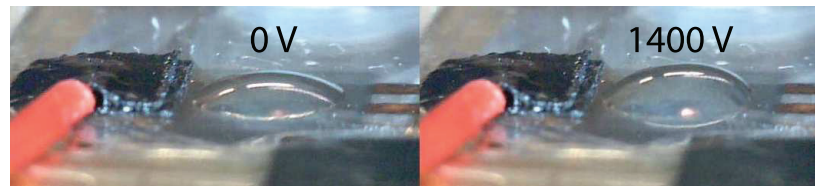
Figure 6.26: Left: picture of a \varnothing 3 mm actuator with a pressure of 950 Pa applied on the membrane's backside, and without applied voltage. Right: picture of the same actuator at 1400 V. With a higher mechanical bias, the spherical cap deformation shape is conserved.
