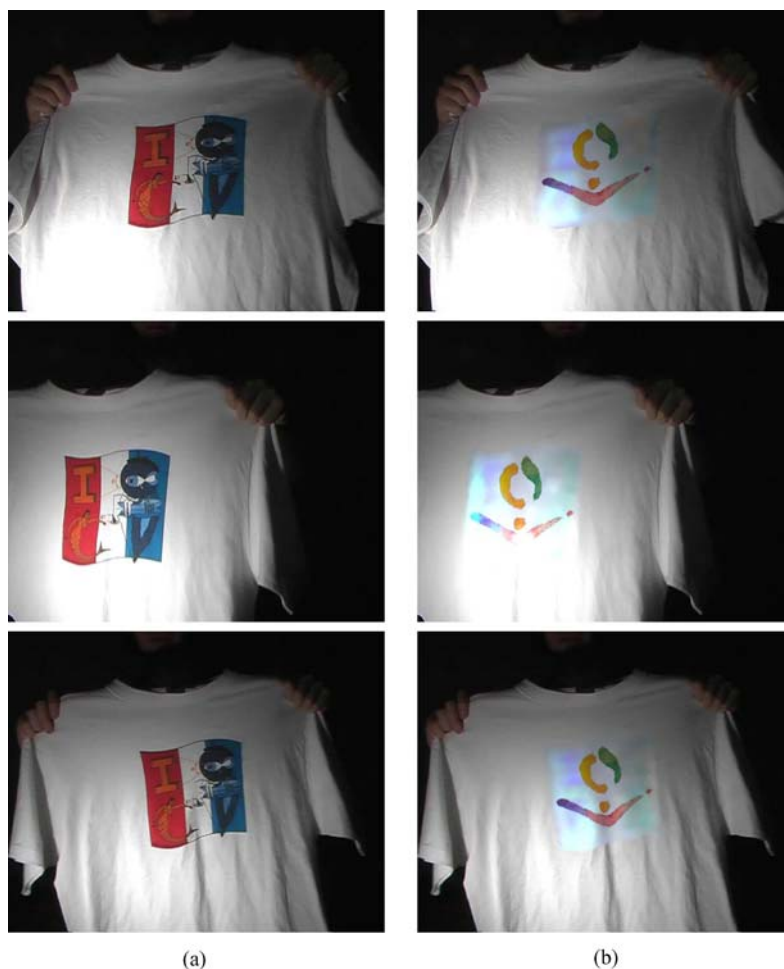
Figure 13. (a) original image. (b) The ISMAR logo replaces the shirt print. Recovering white is hard in this image since the model has large single-colored areas, making light evaluation difficult.
