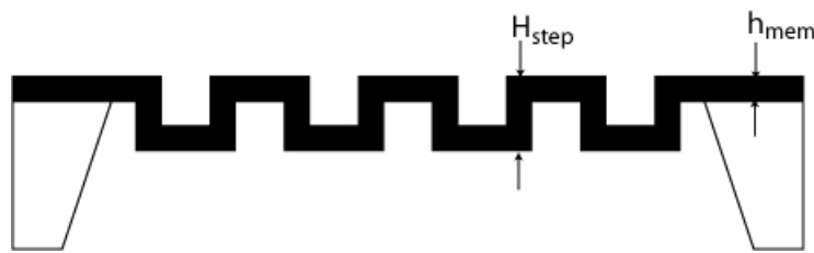
Figure 4: Schematic view of a corrugated membrane of thickness h_{mem} and with a step of corrugation H_{step} .
