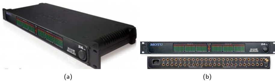
Figure 7.3: MOTU 24I/U audio acquisition card. It has 24 input and 24 output channels, and a possibility to connect 4 MOTU 24I/U cards together.
