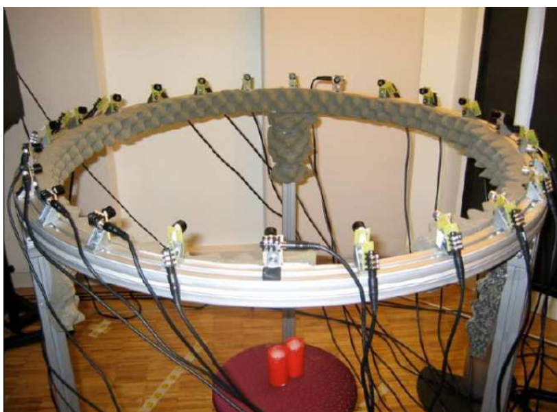
Figure 7.1: Experimental setup. It consists of 12 transmitters and 12 receivers placed on the 1 m radius ring
