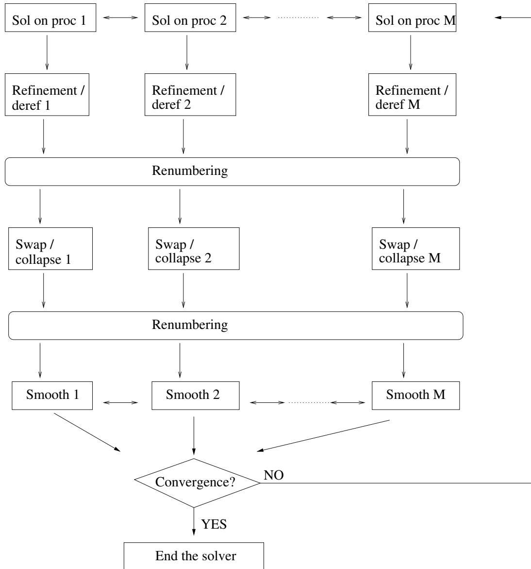
Figure 6.3: Flow-chart for the parallel mesh adaptation.
