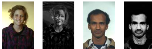
Figure 4: Examples for skin detection. Left: original image, right: results of skin detection. Bright pixels represent high skin probability, dark pixels represent low skin probability. As can be seen skin detection with color histograms yields good results independently of ethnicity.
