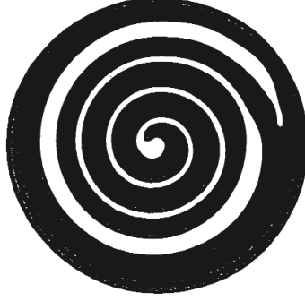
Figure 1.15: Top view of the sidewalls of Trainoff's channel [65]: the white area is the open channel while the walls are in black. The fluid enters through a hole in the center of the bottom plate and exits through a hole on the periphery after having traveled through the inlet (the small width channel part located in the center), the nozzle and eventually the working section of the channel.
