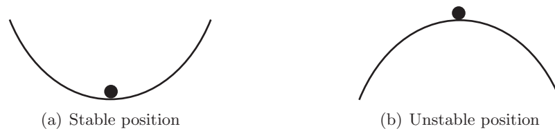
Figure 1.7: A stable position subjected to a perturbation will return to its initial state.
