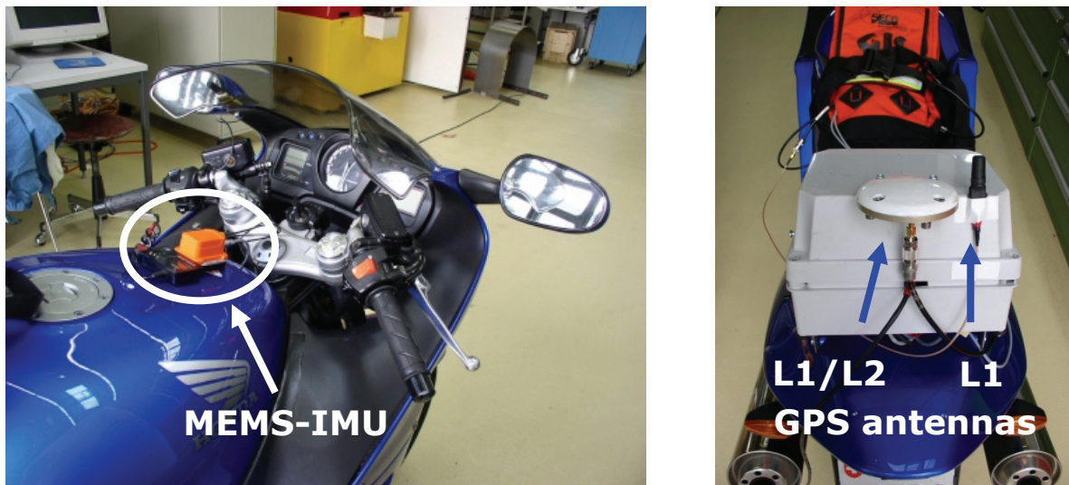
Figure 1 : GPS/MEMS-IMU system setup
