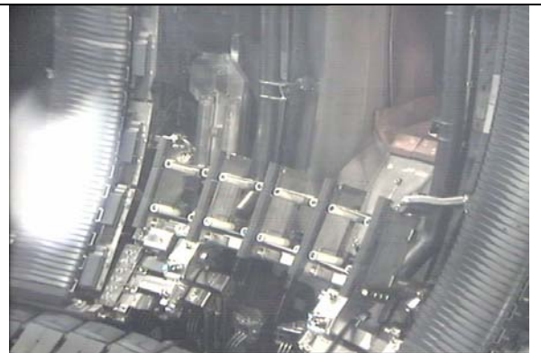
Figure 1. View of one group of four AE antennas as installed in vessel during June 2005.
