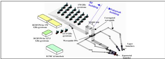
**FIGURE 1.** Overall ITER EC system (as described in Ref. [1]) comprised of power supplies, two gyrotron types, transmission lines and two launcher types.
