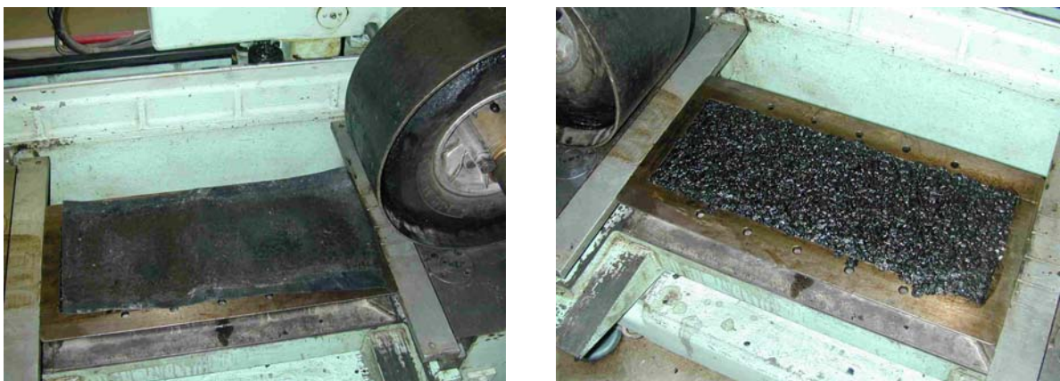
Figure 10. 4 : Final stage of compaction (left) and the sample (right)
