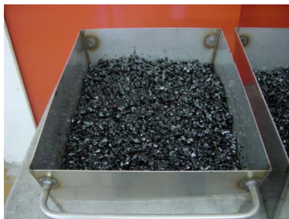
Figure 9. 3 : Mix AG4 prepared in a metal pan for aging
