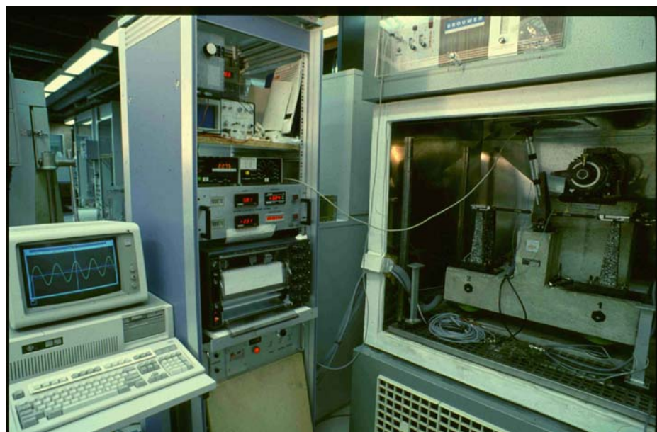
Figure 9. 13 : Two point bending equipment at LAVOC
