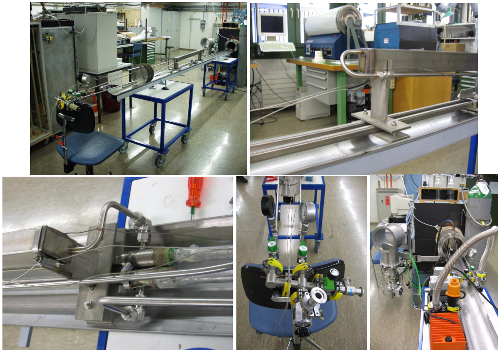
Figure 10: Top left: Solder test assembly before insertion into furnace. Top right: Solder reservoir with pumping port. Bottom left: (top) and outlet (bottom) into cable sample. On the right side are the sealed joints., Bottom middle: Plumbing: bottom: pumping port; Right: Line to Argon. Setup shown does not correspond exactly to final version as shown in schematic. Bottom right: Complete assembly mounted into furnace.
