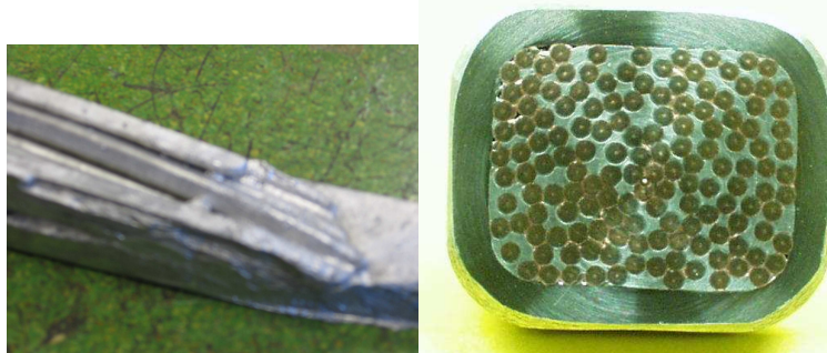
Figure 11: Left: Partially melted solder bars. Right: Result of solder-filling of SUBSAM I cable.
