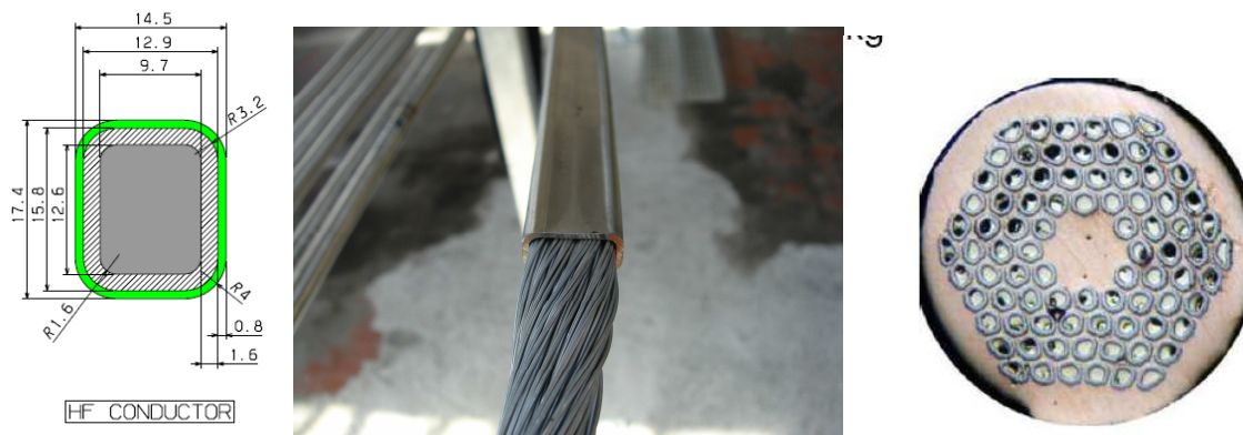
Figure 1: Example of a prototype for the EFDA dipole high field cable. Left: jacket dimensions, Middle: photo during jacketing (photo taken is from a similar but not identical conductor), Right: strand.
