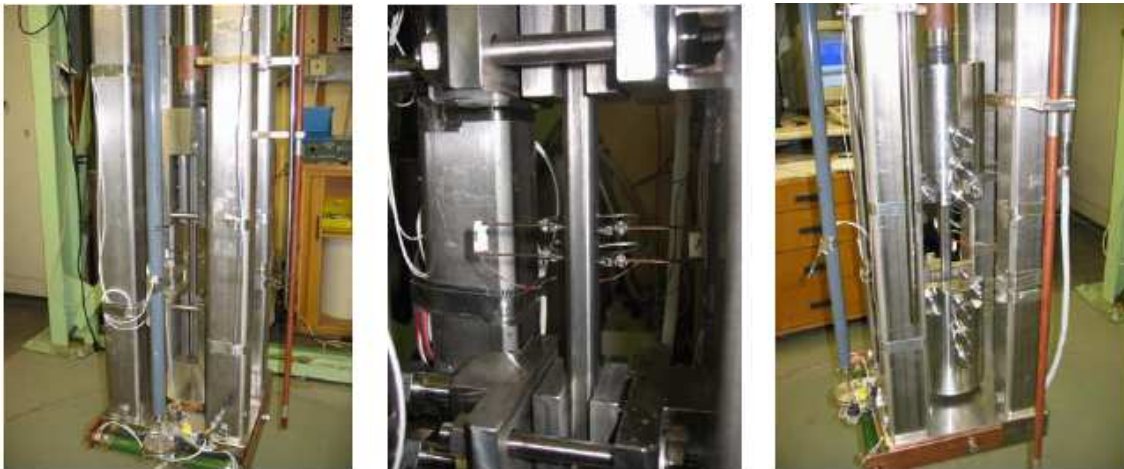
Figure 20: Soldered Cable Sample mounted into the test-rig: Left Cryostat insert, Middle: Force grips with sample, Right: Test Insert before insertion in cryostat.
