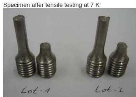
Figure 17: BiSn solder specimen after testing at FZK.
