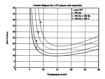
Fig.2: Confinement capability needed to sustain steady DT burning in plasmas having flat pressure and temperature profiles for various concentrations of impurities. The confinement capability tE is in bar.s. and the volume averaged pressure is the total plasma pressure.
