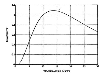
Fig.1: The reactivity of a 1:1 DT plasma, R(T) as function of temperature expressed in keV.
