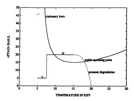
Fig.3: Schematic representation in the (\tauE,T) plane of a possible approach to a steady burn operating point (\*), assuming a soft degradation of the confinement near the pressure limit. The stationary burn curve is the case with 5% He + 3% Be. L and H refer to the L and H-regimes respectively.
