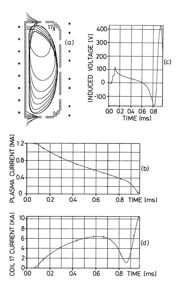
Fig. 5. (case 1051) rapid current loss and vertical disruption; (5a) snapshots of the outermost flux surface; (5b) plasma current; (5c) the induced voltage at a point 25 mm below the center of the fast coil; (5d) the induced current in the short circuited fast coil.
