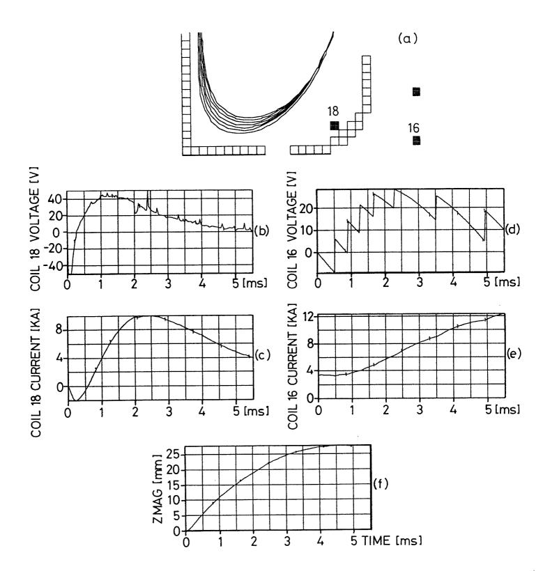
Fig. 4. (case 950) plasma control of programmed plasma motion with both fast and slow coils; (4a) plasma and coil geometry, where snapshots of the lower portion of the outermost flux surface show the bottom of the plasma moving upwards; (4b) the bottom fast coil voltage and (4c) resulting fast coil current; (4d) voltage and (4e) current on the bottom shaping coil at large major radius; (4f) the vertical position of the magnetic axis.
