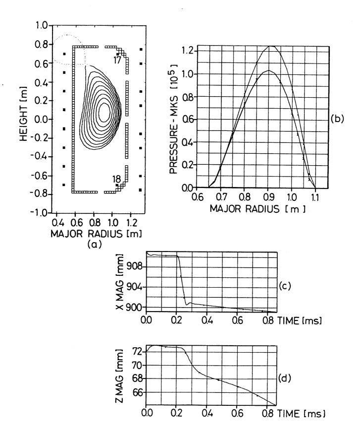
Fig. 1. (case 940) plasma response in the absence of feedback; (1a) a 2.2/1 elongated, single-null divertor equilibrium in TCV geometry. (1b) before and after radial profiles of pressure; (1c) radial and (1d) vertical time response of the position of the plasma magnetic axis.
