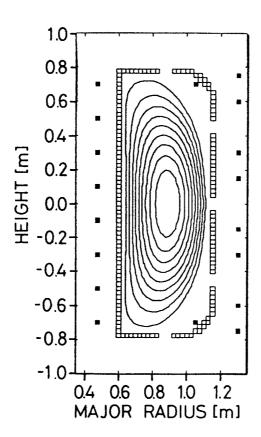
Fig. 3. (cases 915,950) initial MHD equilibrium with  $\kappa$ =3/1 and  $l_p$  = 1200 KAmps calculated with TSC for studying control of programmed motion.
