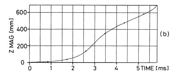
Fig. 6. (case 1060) slow, non-symmetric disruption; (6a) plasma current; (6b) vertical position of the magnetic axis.
