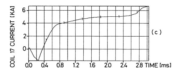
Fig. 2. (case 943) feedback control using only rapid coils.  $\beta$  is dropped from 5.8% at to 5.3%; (2a) vertical position of the magnetic axis versus time; (2b) the applied voltage and (2c) resulting current waveforms of the upper feedback coil.
