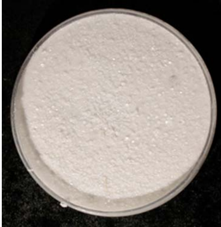
Figure I. IV: Surface in contact with water of the alite at 28 days of chemical shrinkage measurement (in an erlenmeyer flask)
