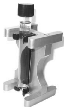
Figure 1.4 Standard setup for the magnetic separation. The magnetic particles in solution are attracted towards a permanent magnet and the liquid is extracted from the vial.
