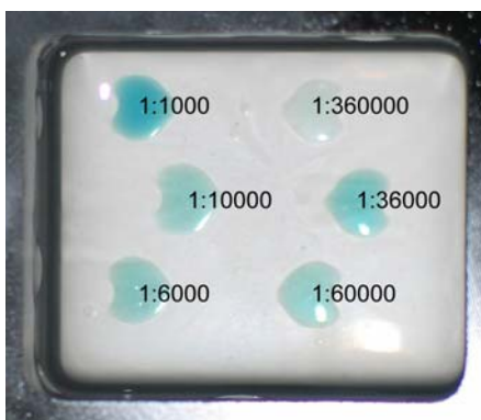
Figure 5.15 Photograph of the chromogen droplets after the reaction with different concentrations of enzyme-labeled antibody. The incubation time was 15 min. (The dilution ratio 1:1000 corresponds to a concentration of 1300 ng/ml).
