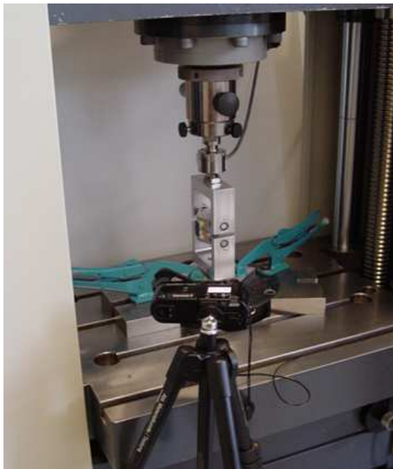
Figure 3.3 and 3.4: Set-up for tension and compression tests: the lower piling is rigidly fixed, the upper is mobile and contains the load cell; the test blocks are mounted in a bearing perpendicular to the sense of the applied force
