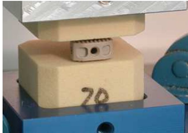
Fig. 3.51: Set-up for the subsidence test; the lower foam block is rigidly fixed; the upper one is on the actuator and connected with the load cell
