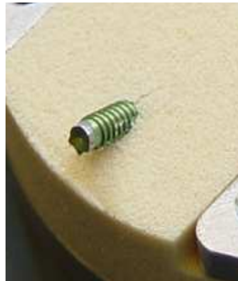
Fig. 3.32: Test 017, broken screw; SynFix-C 015 2.4/16
