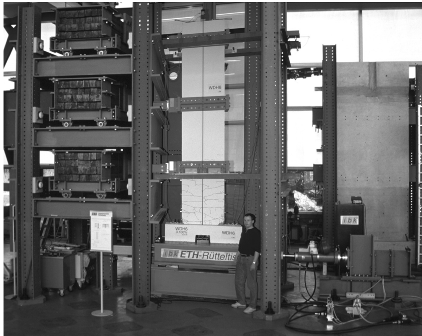
Fig. 3. Test set-up with wall WDH6 [1].
