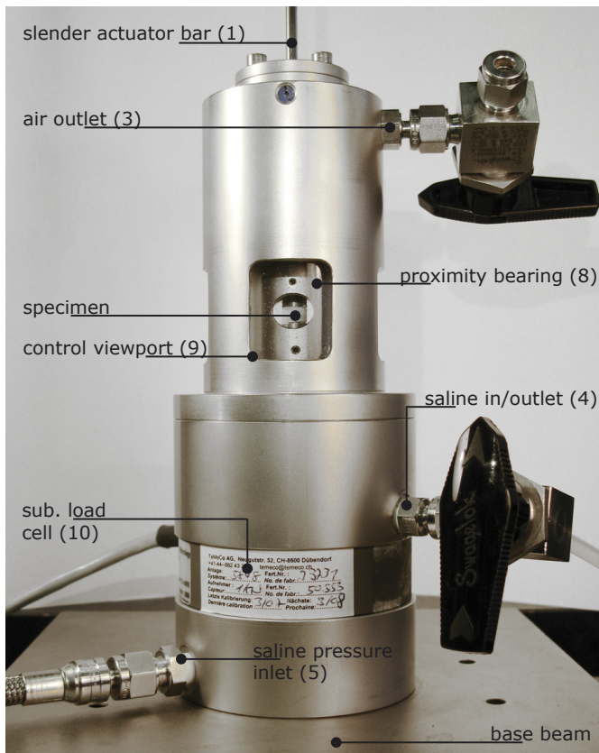
Figure 4.9: Photograph of the custom made pressure chamber (see figure 3.8 for details).
