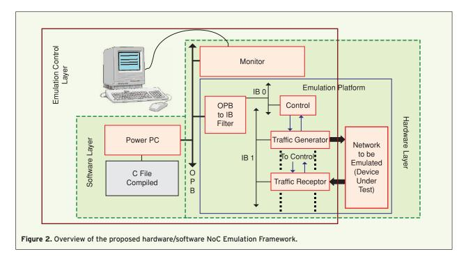
tem on NoCs. Then Chan et al. [11] present a mixed VHDL/SystemC implementation and simulation methodology, which employs a template router to support several interconnection networks. These previous approaches enable a fast exploration of various features of NoCs, but their level of accuracy is limited. Furthermore, their simulation speed is still lower than our proposed emulation framework.
