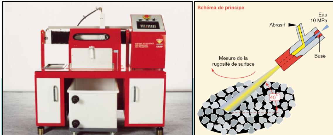
Figure 3: Machine *GRAP* – principe (source: www.lcpc.fr)
