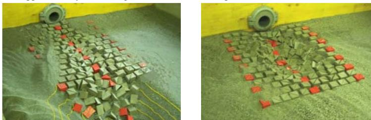
Figure 9: Location of scour hole as a function of tailwater level for  $Q = 12.5$  l/s; high tailwater  $h_{TW} = 10.9$  cm (left), low tailwater  $h_{TW} = 1.9$  cm (right)
