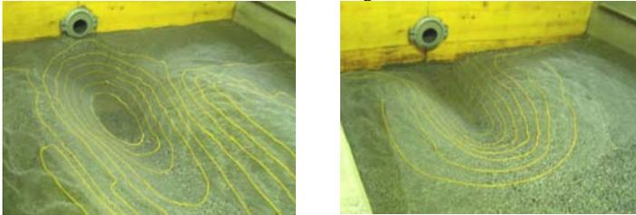
Figure 5: Scour hole for  $D = 10$  cm and  $Q = 12.5$  l/s; high tailwater  $h_{TW} = 10.9$  cm (left), low tailwater  $h_{TW} = 1.9$  cm (right)
