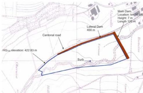
Figure 8. Retention basin at Lengnau layout
