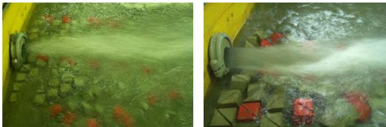
Figure 3:  $Q = 21.5$  l/s; high tailwater, prism size 5 cm and  $h_{TW} = 11.6$  cm (left), low tailwater, prism size 8 cm and  $h_{TW} = 3$  cm (right)
