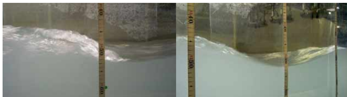
Figure 6.12: Stationary wave at the end of the bend with surface roller (left) and a common one (right). Picture taken across the outer side wall
