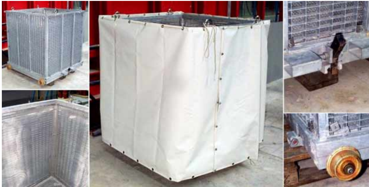
LEFT-TOP: Structure of the filtering basket, LEFT-BOTTOM: view from inside, CENTER: Basket with the skirt, RIGHT TOP: Closing mechanism, RIGHT-BOTTOM: wheel and back flap
