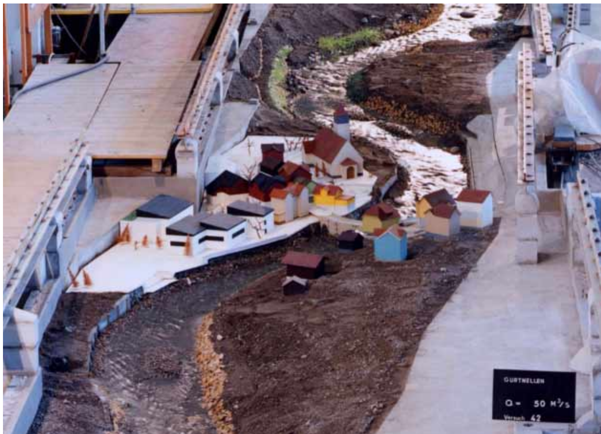
Figure 1.1: Hydraulic scale model of the Reuss River, Gurtellen, Switzerland [Kuster et al., 1992]
