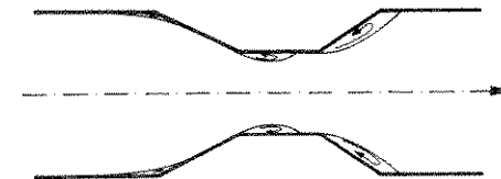
Figure 28 : Flume with broken plane transitions and resulting separation zones (schematically).
