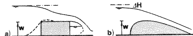
Figure 17 : Weirs of equal height w in a rectangular channel having identical flow conditions, a) broad-crested weir with separation zones at the upstream leading edge and b) airfoil weir having gradually varied bottom geometry and no separation zones. Under equal discharge, the upstream flow depth is higher ( \Delta h ) in case a) than in b).
