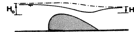
Figure 31 : Notation for submerged flow conditions. All parameters are measured vertically from the spillway crest.
