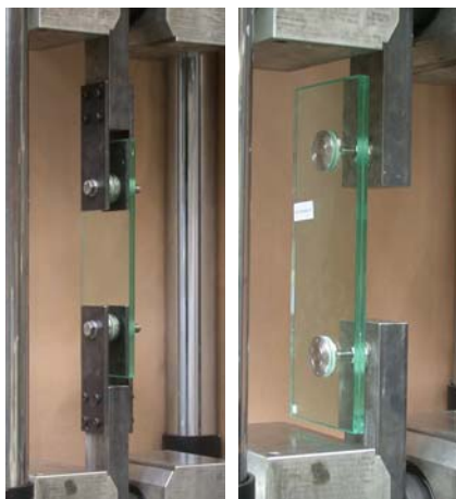
Figure 3 and Figure 4 Specimens in the testing machine - axially and eccentrically applied load
